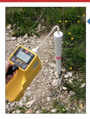
Multi-gas meter used to measure concentrations of Methane, CO2, and other gases in well
