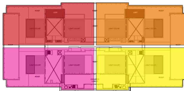
Figure 3.1 - Phasing diagram showing ideal quadrant divisions
