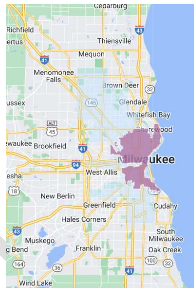
Figure 8. The City of Milwaukee maintains a large combined sewer system (purple), which can lead to sewerage mixing with stormwater runoff during extreme precipitation events. Source: Reflo 2023.
