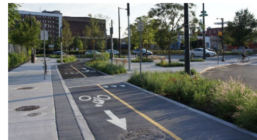
EXAMPLE OF A SHARED-USE PATH WITH DEPRESSED STORMWATER BASIN
