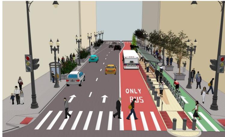
Chicago's planned Central Loop BRT service will operate in dedicated bus lanes and include protected green bicycle lanes on three streets.
