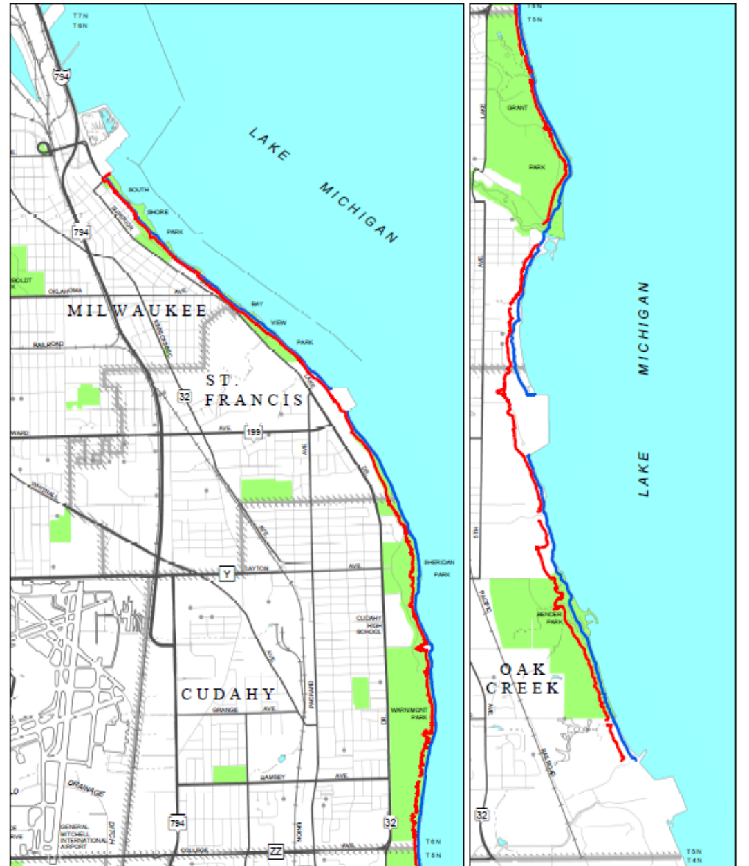
— BLUFF CREST — BLUFF TOE ■ MILWAUKEE COUNTY OWNED PROPERTY Note: (Based on 2015 Lidar Topo but aligned in various locations to data provided to SEWRPC by Wisconsin Coastal Management Program) Source: Wisconsin Coastal Management Program and SEWRPC
