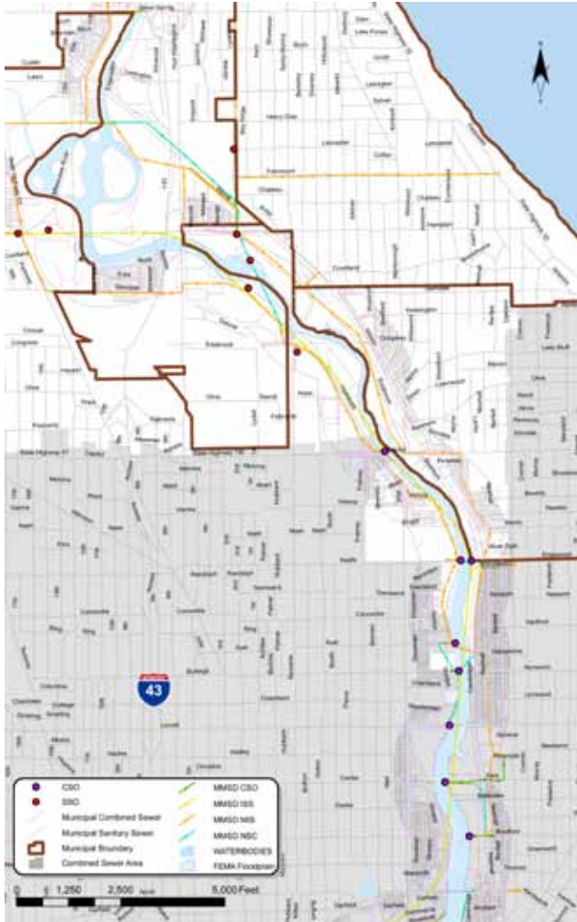
MMSD SERVICE AREA SEWER MAP (2008) Study area contains 7 sanitary sewer outfalls and 8 combined sewer outfalls that can discharge sewage during wet weather events.
