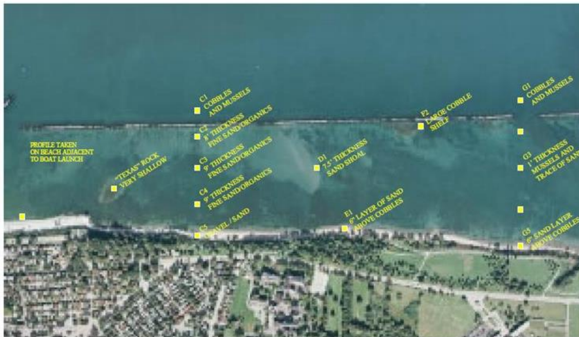
Figure 4.2: Historical Jet Probe Locations (center segment)
