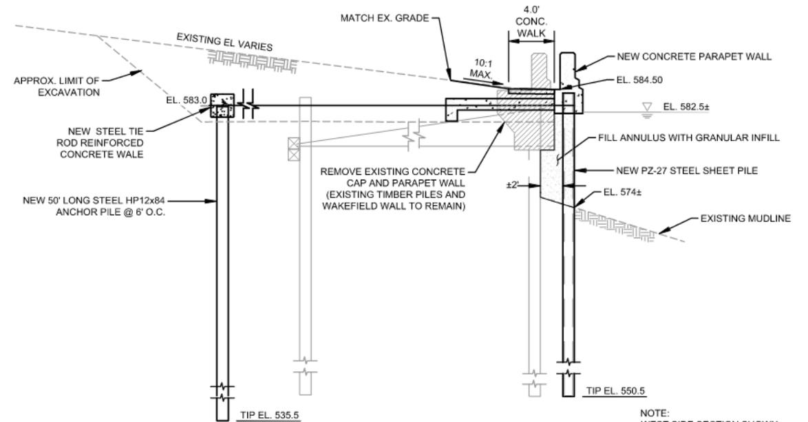
C401 **C** PROP. CONCRETE PARAPET WALL SECTION
