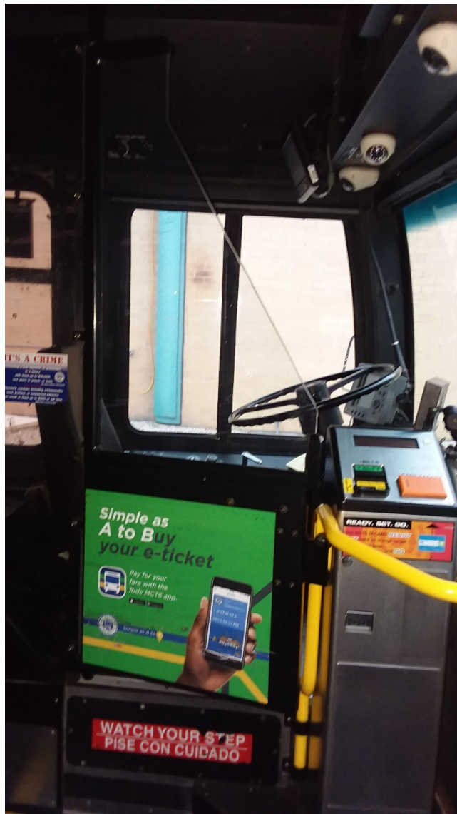
Photo: 1 st Generation Shield by Bentech Co. still installed on 177 buses
