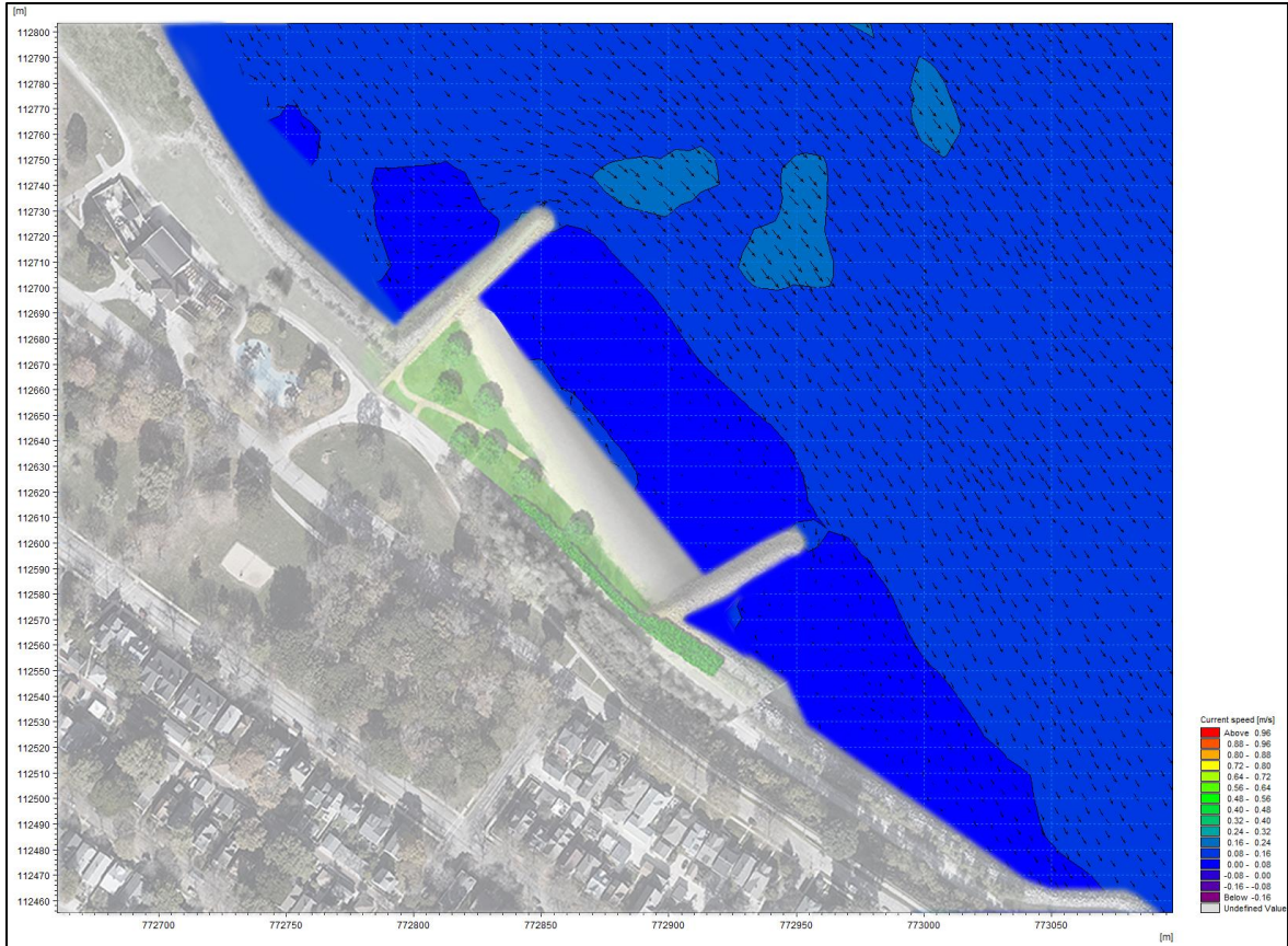
Figure 43: Current Speeds caused by winds from the NNE 1year return period event (Alternative 2).
