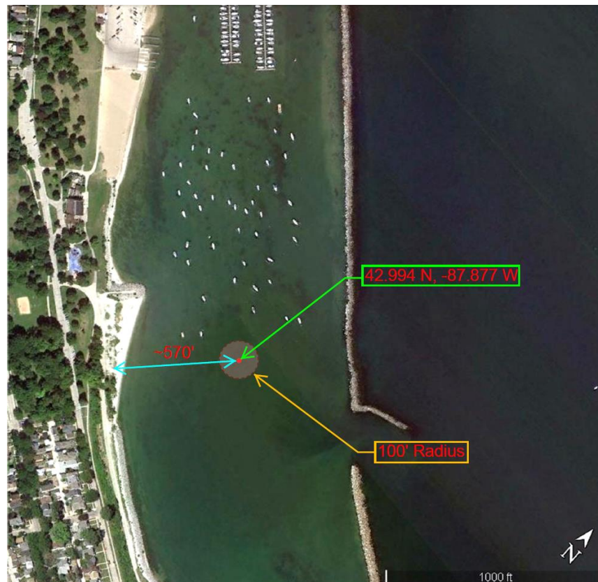
Figure 9: Position of the deployed ADCP behind the breakwater entrance.
