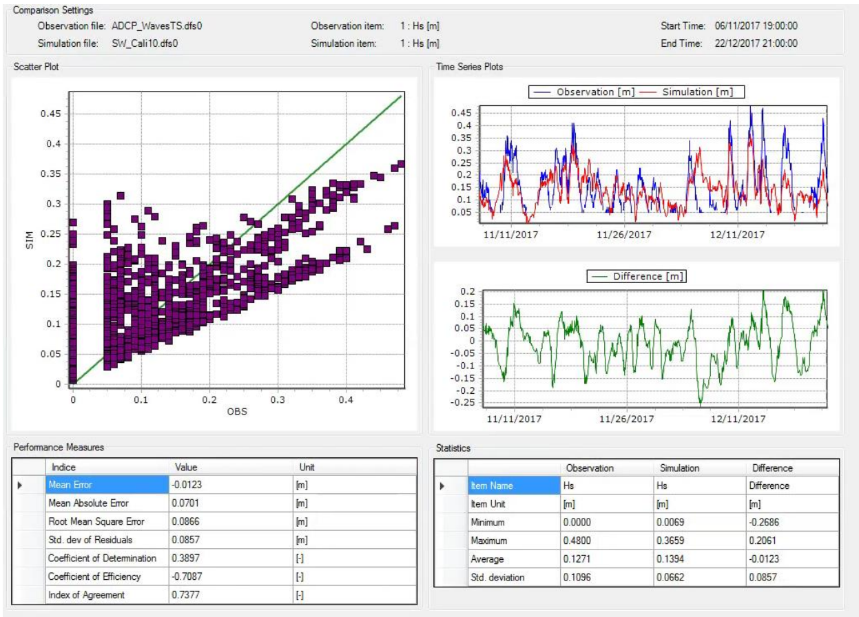
Figure 32: Comparison between the ADCP measured wave heights and the model simulation after the tuning parameters were changed.
