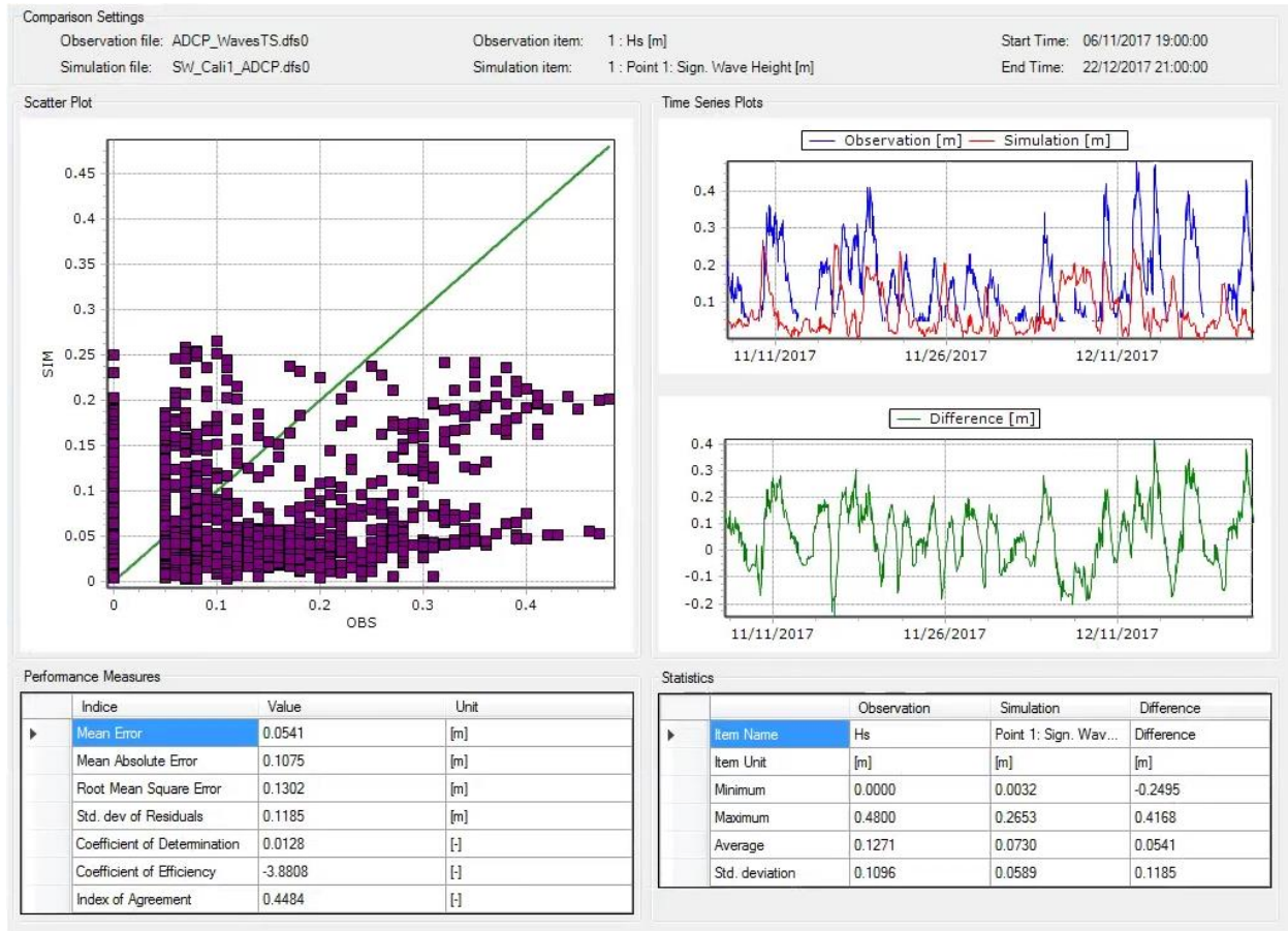
Figure 31: Comparison between the ADCP measured wave heights and the model simulation using the default parameters.
