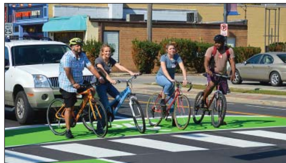
A bike box along North Avenue improves bicyclist safety and enhances Wauwatosa's multi-modal transit initiatives. Source: Ayres Associates
