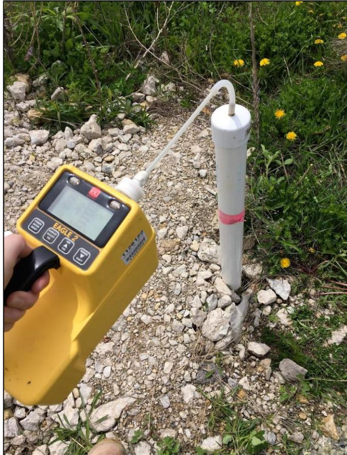
Multi-gas meter used to measure concentrations of Methane, CO<sub>2</sub>, and other gases in well
