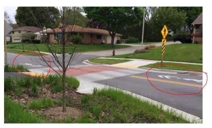
Other construction methods include colored asphalt, thermoplastic markings, and textured pavement. Each of these is more expensive than paint, and therefore should be evaluated according to the site needs and available budget.
