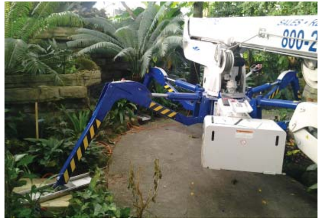
Specialty lift used to maintain the Domes
