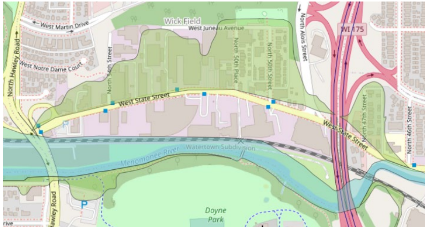
Figure 13. Flooding along West State Street corridor, indicated by 100-year and 500-year flood zones.
