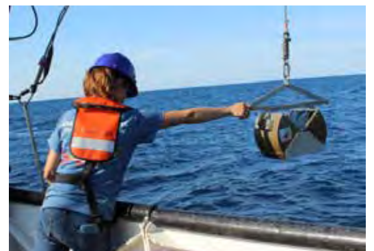
Large research vessels allow scientists to test water quality and the health of bottom sediments near the coastline and far offshore. Cylindrical, multi-chambered “Rosette” samplers are used to collect water. Small metal “Ponar” samplers are used to scoop up and retrieve sediments.
