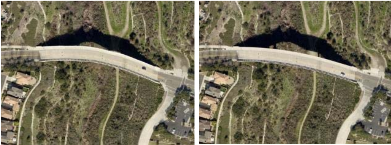
Before and After Bridge Correction
